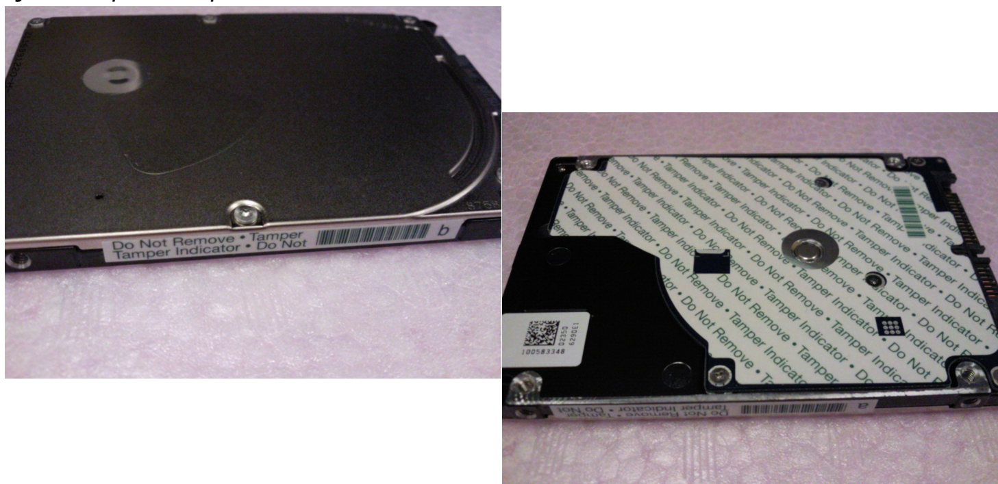
Figure 6 Example of FIPS tamper evidence labels.
