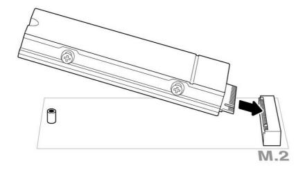
8. Hold down FireCuda 530R SSD while you fasten the mounting screw. Make sure the SSD is secured in place.
